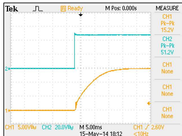
Figure 123: AEE01CC36-L Output Voltage Startup Characteristic by Vin Vin = 48Vdc Load: Io = ±1.33A Ch 1: Vo Ch 2: Vin
