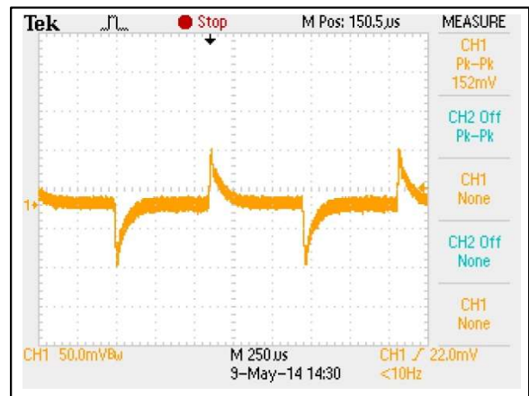
Figure 22: AEE03B18-L Transient Response Vin = 24Vdc Load: Io = 100% to 75% load change Ch 1: Vo
