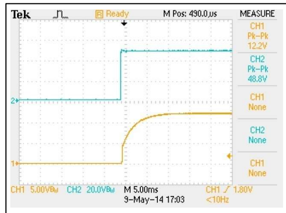
Figure 87: AEE03B36-L Output Voltage Startup Characteristic by Vin Vin = 48Vdc Load: Io = 3.33A Ch 1: Vo Ch 2: Vin
