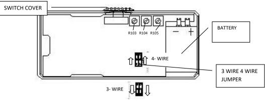
Figure 3. 3-Wire/4-Wire Jumper Location
