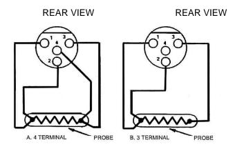
Figure 2. 100 Ohm Platinum RTD Connections
