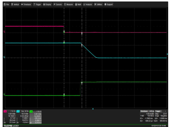
Figure 6: LCM1500L-T-4 Turn Off Characteristic via INH_EN Load: lo = 125A (12V), lsb = 2A (5V) Ch 2: INH_EN Ch 3: Vo Ch 4: G_DCOK_C
