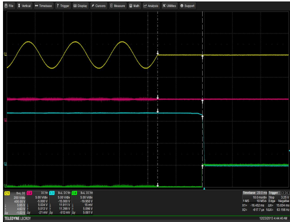
Figure 3: LCM1500L-T-4 Hold-up Time Vin = 90Vac / 47Hz / 0° Load: lo = 125A (12V), lsb = 2A (5V) Ch 1: Vin Ch 2: Vsb Ch 3: Vo Ch 4: G_DCOK_C
