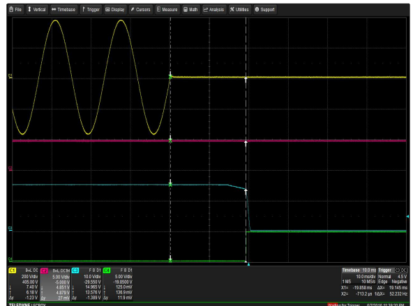
Figure 15: LCM1500N-T-4 Hold-up Time Vin = 264Vac / 60Hz / 0° Load: lo = 100A (15V), lsb = 2A (5V) Ch 1: Vin Ch 2: Vsb Ch 3: Vo Ch 4: G_DCOK_C
