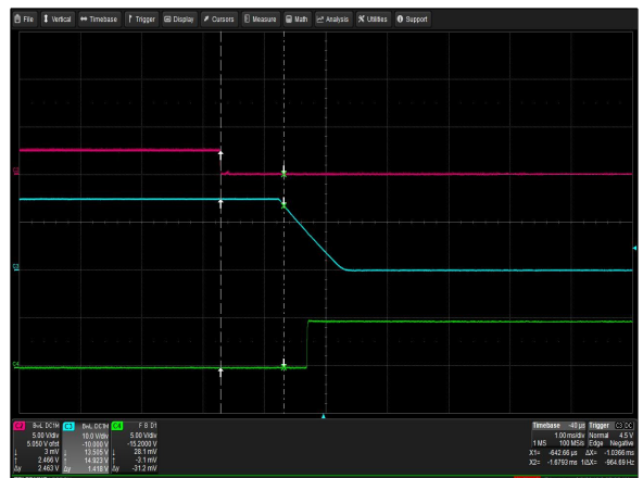
Figure 17: LCM1500N-T-4 Turn Off Characteristic via INH_EN Load: lo = 100A (15V), lsb = 2A (5V) Ch 1: INH_EN Ch 2: Vo Ch 3: G_DCOK_C
