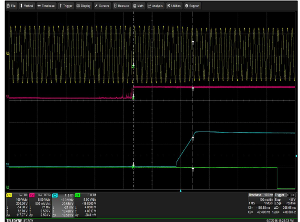
Figure 13: LCM1500N-T-4 Turn-on delay via INH_EN Vin = 90Vac Load: lo = 100A (15V), lsb = 2A (5V) Ch 1: Vin Ch 2: INH_EN Ch 3: Vo Ch 4: G_DCOK_C
