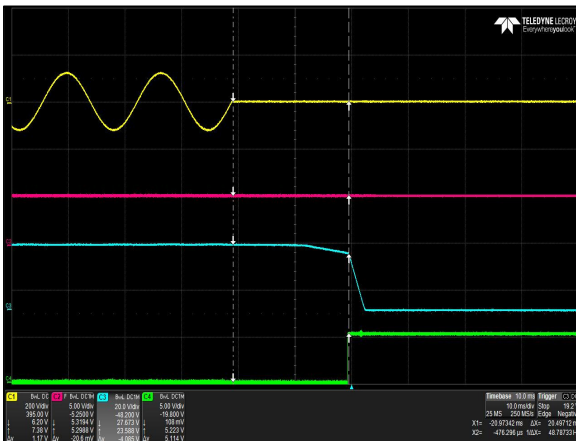
Figure 36: LCM1500R-T-4 Hold-up Time Vin = 90Vac / 47Hz / 0° Load: Io = 53.6A (28V), Isb = 2A (5V) Ch 1: Vin Ch 2: Vsb Ch 3: Vo Ch 4: G_DCOK_C
