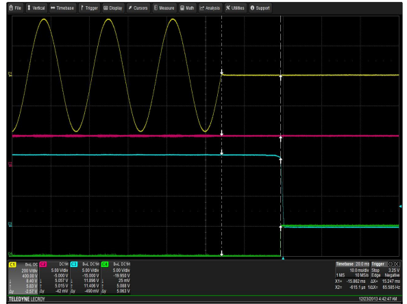
Figure 4: LCM1500L-T-4 Hold-up Time Vin = 264Vac / 60Hz / 0° Load: lo = 125A (12V), lsb = 2A (5V) Ch 1: Vin Ch 2: Vsb Ch 3: Vo Ch 4: G_DCOK_C
