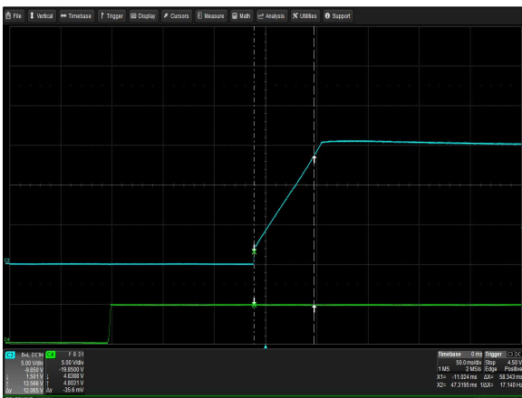
Figure 16: LCM1500N-T-4 Output Voltage Startup Vin = 90Vac Load: lo = 100A (15V), lsb = 2A (5V) Ch 1: Vo Ch 2: G_DCOK_C
