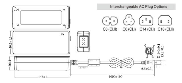
DC Cable: UL1185 16AWG 1000 mm with ferrite core Connector: #03 - 2.5 x 5.5 x 9.5 mm, fork type, 18 to 52 V #49 - 4PIN (Keycon equal), 12 to 17 V
