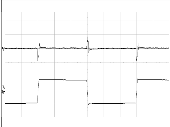
Figure 7: AGQ200B-48S3V3 Transient Response (1mS/div) 25%~50%~25% load change, 0.1A/uS slew rate Ch 1: Vo (50mV/div) Ch 2: Io (10A/div)
