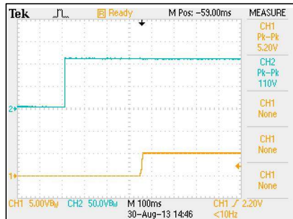
Figure 42: ERM15A110 Output Voltage Startup Characteristic by Vin Vin = 110Vdc Load: Io = 15A Ch 1: Vo Ch 2: Vin
