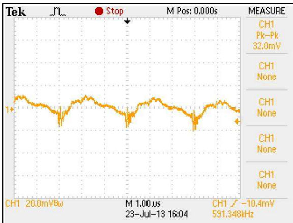
Figure 30: ERM03H72 Typical Output Ripple and Noise. Vin = 72Vdc Load: Io = 3.125A Ch 1: Vo
