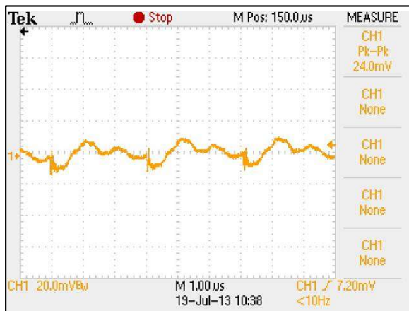
Figure 48: ERM06B110 Typical Output Ripple and Noise. Vin = 110Vdc Load: Io = 6.25A Ch 1: Vo
