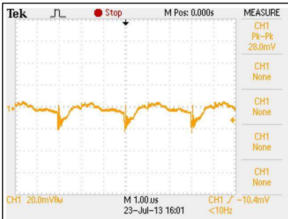
Figure 12: ERM06B72 Typical Output Ripple and Noise. Vin = 72Vdc Load: Io = 6.25A Ch 1: Vo
