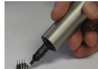
Figure 1: IC Pin Voltage Measurement
