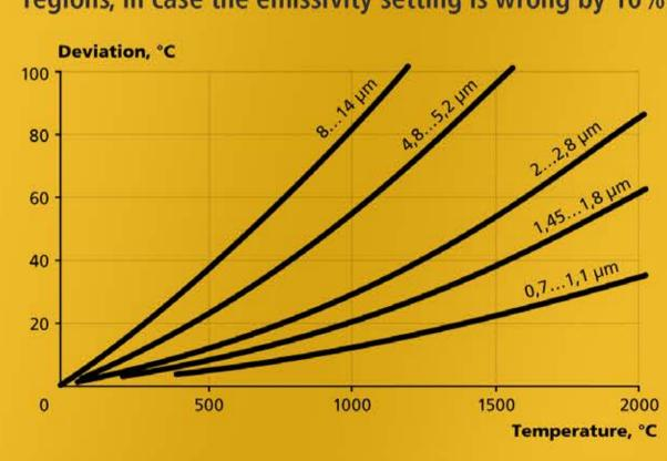
To minimize systematic measuring errors, which may be caused by external influences (e.g. surface variations, reflections), temperatures on metal surfaces should always be measured at the shortest possible wavelength.
