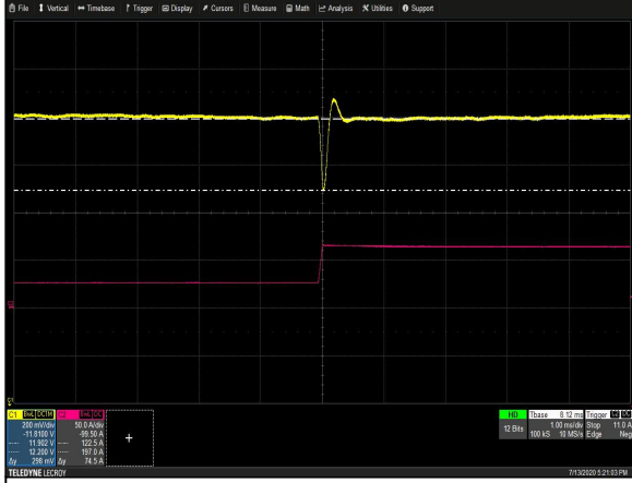
Figure 10: CSU800AP-3-600 Transient Response - V O Deviation 40% to 100% load change 0.5 A/uS slew rate Vin = 230 Vac Ch 1: V O Ch 2: I O
