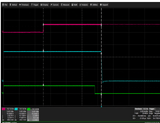
Figure 9: DS2400SPE-3 Turn Off Characteristic via PSON V_{in} = 90V_{ac} Load: I_o = 114.8A I_{SB} = 3.5A Ch 2: PSON Ch 3: V_o Ch 4: PWOK
