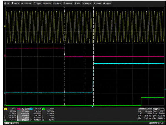
Figure 2: DS2400SPE-3 Turn-On Delay via PSOn Vin = 90Vac Load: I_o = 114.8A I_{SB} = 3.5A Ch 1: AC Mains Ch 2: PSOn Ch 3: V_o Ch 4: PWOK
