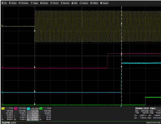
Figure 1: DS2400SPE-3 Turn-On Delay via AC Mains Vin = 90Vac Load: I_o = 114.8A I_{SB} = 3.5A Ch 1: AC Mains Ch 2: V_{SB} Ch 3: V_o Ch 4: PWOK
