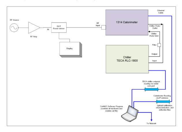
Figure 18: Manual RF Calibration Set-up
