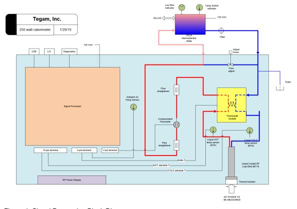
Figure 4: Signal Processing Block Diagram
