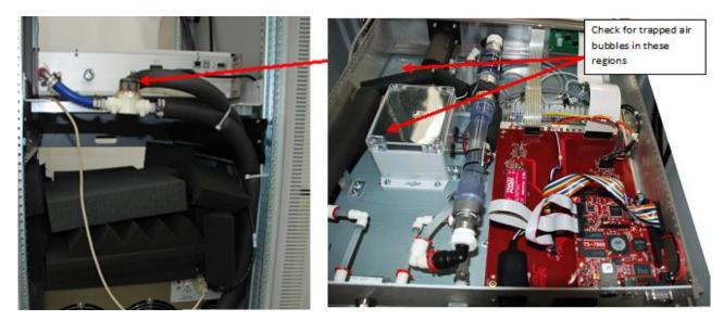
Figure 11: Look for trapped air bubbles
