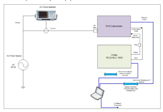
Figure 17: Manual AC Calibration Configuration
