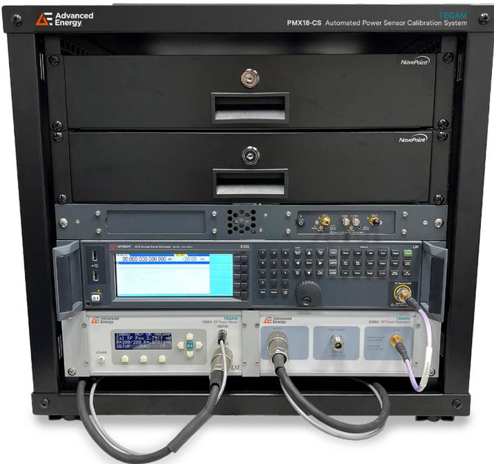
**Ready to Work:** The PMX18-CS comes packaged with everything necessary to calibrate reflection and cal factors for 9 kHz to 18 GHz power sensors. The system includes an RF standard, RF power meter, RF signal source, VNA, plus an assortment of accessories to increase your calibration capability.
