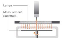
Measurement in Lamp Heated Reactor
