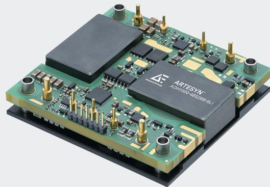
Advanced Energy's Artesyn ADH1300-48S28 series is a single output DC-DC converter with standard half-brick outline and pin configuration. It provides a regulated low noise output and function for a digital-controlled PMBus interface. It delivers up to 1300 W with 28 VDC output voltage. The 95.5% peak efficiency and excellent thermal management, and operational ambient temperature range of -40°C to +85°C makes it an ideal choice for use in datacom and telecommunication applications.
