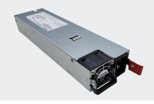
Advanced Energy's Artesyn CSU front end series is designed to provide a flexible power conversion solution for compute, storage, and networking equipment in the common redundant power supply (CRPS) form factor. This series of AC-DC products is housed in the industry standard 1U x 73.5 mm x 265 mm CRPS form factor. Featuring a power rating of 3200 W, the series can cover power hungry applications where there are space constraints.
