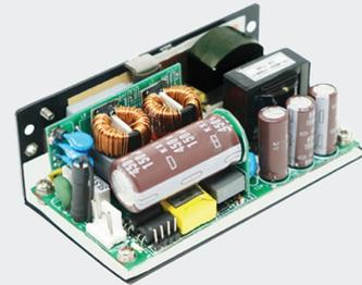
Advanced Energy's SL Power NCF250 CF rated\* medically approved AC-DC power supplies are available with a nominal main output of 12 V, 15 V, 24 V, or 48 V. NCF250 series power supplies provide up to 250 W of output power with air flow. All models have output overvoltage, short circuit and overload protection and a 2.4 x 5.0 x 1.6 inch form factor.
