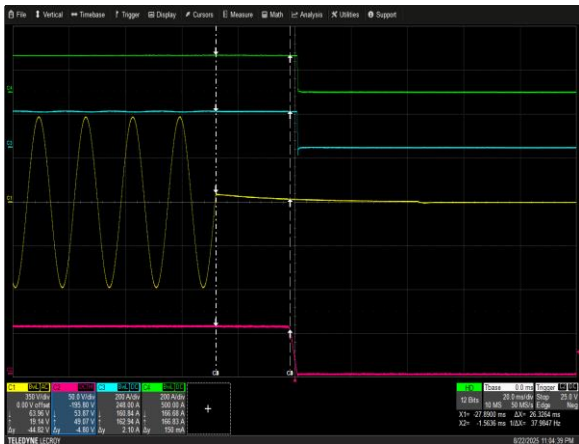
Figure 3: FCM30K Hold-up Time Vin = 408VAC Load: Io = 330A Ch 1: Vin Ch 2: Vo Ch 3: Io 1 Ch 4: Io 2
