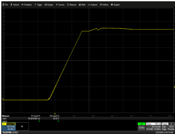
Figure 5: FCM30K Turn-on Overshoot Vin = 480VAC Load: Io = 551A Ch 1: Vo
