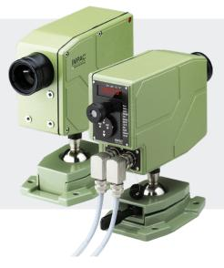
The Impac<sup>®</sup> IS 12-AI is a version of the pyrometer IS 12, specially designed for the measurement of aluminum. The robust die-cast housing with protection class IP 65 is designed for the use in industrial environments. The parameters of this digital instrument can be set directly via push buttons on the rear side of the instrument. The built-in digital display indicates the corresponding parameters or the actual temperature reading in measuring mode.
