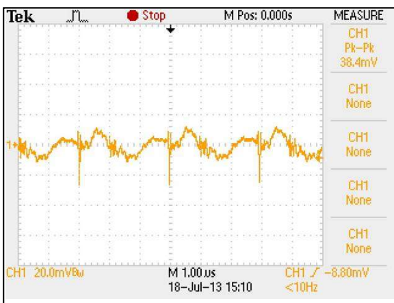
Figure 12: ERM04B72 Typical Output Ripple and Noise. Vin = 72Vdc Load: Io = 4.17A Ch 1: Vo
