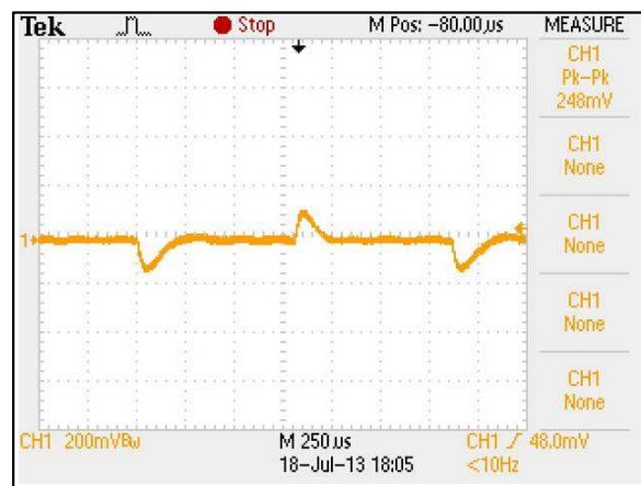
Figure 4: ERM10A72 Transient Response Vin = 72Vdc Load: Io = 100% to 75% load change Ch 1: Vo
