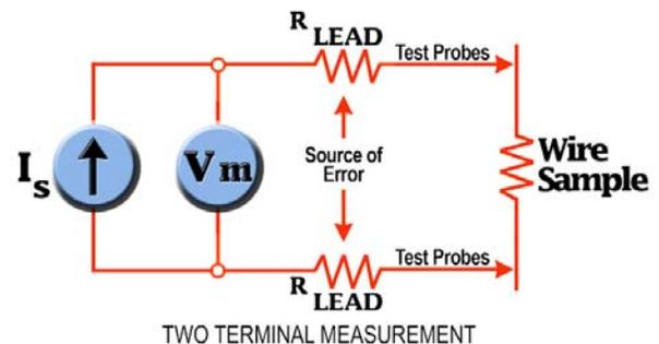
Figure 1 – The measurement method known as the 2-terminal method is subject to error introduced by  $R_{LEAD}$ .
