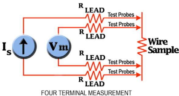
Figure 2 – The 4-terminal method is widely recognized as the preferred form of measurement.
