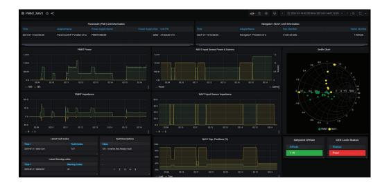
Example custom dashboard for monitoring match network and RF generator data with Smith chart:
