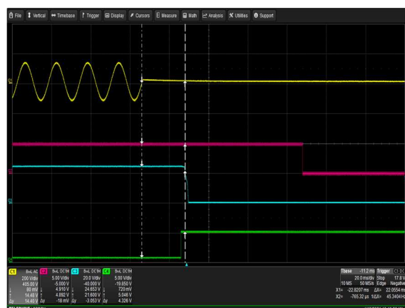
Figure 21: μMP10T-S2Q-S2Q-S2Q-S2Q-S2Q-90-A Hold-up Time via AC mains V_{in} = 90V_{ac}/63Hz Load: I_O = 41.66A I_{SB} = 2A Ch 1: AC Mains Ch 2: V_{SB} Ch 3: V_O Ch 4: Global DCOK
