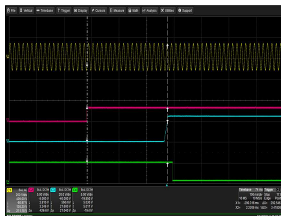
Figure 20: μMP10T-S2Q-S2Q-S2Q-S2Q-S2Q-90-A Turn-on delay via Global inhibit V_{in} = 90V_{ac} Load: I_O = 41.66A I_{SB} = 2A Ch 1: AC Mains Ch 2: Global inhibit Ch 3: V_O Ch 4: Global DCOK
