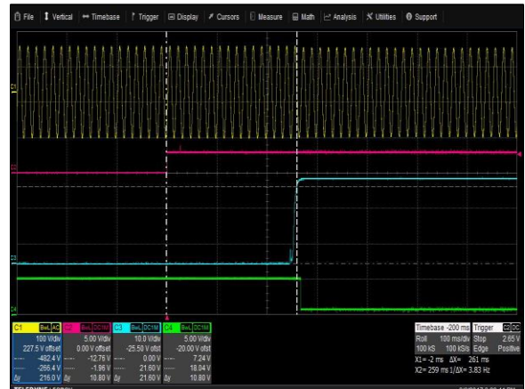
Figure 11: µMP09T-SKQ-S2Q-30-A Turn-on delay via Global inhibit Vin = 90Vac Load: I_O = 23A I_{SB} = 2A Ch 1: AC Mains Ch 2: Global inhibit Ch 3: V_O Ch 4: Global DCOK
