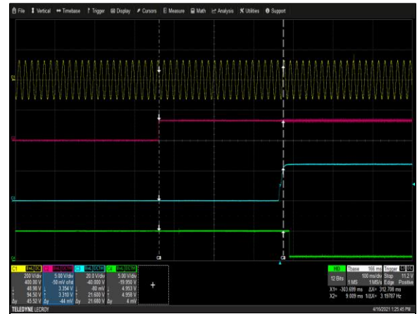
Figure 31: μMP16C-SKQ-SKQ-30-A Turn-on delay via Global inhibit Vin = 90Vac Load: I o = 41.66A I SB = 2A Ch 1: AC Mains Ch 2: Global inhibit Ch 3: V O Ch 4: Global DCOK
