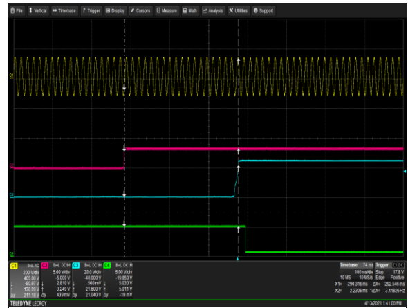
Figure 20: µMP10T-S2Q-S2Q-S2Q-S2Q-S2Q-S2Q-90-A Turn-on delay via Global inhibit Vin = 90Vac Load: I O = 41.66A I SB = 2A Ch 1: AC Mains Ch 2: Global inhibit Ch 3: V O Ch 4: Global DCOK
