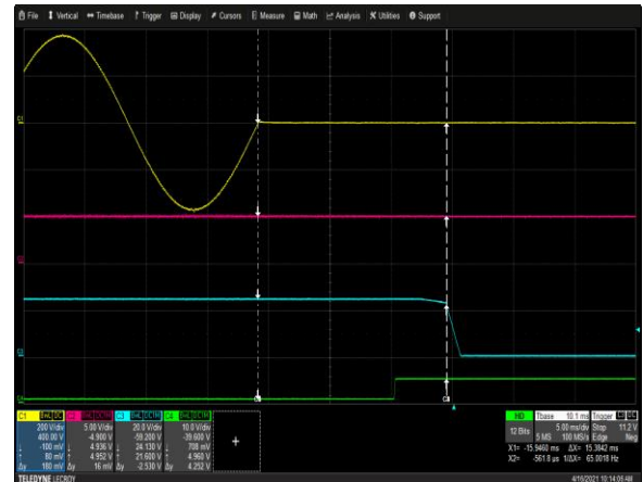
Figure 33: μMP16C-SKQ-SKQ-30-A Hold-up Time Vin = 264Vac/47Hz Load: I o = 75A I SB = 2A Ch 1: AC Mains Ch 2: V SB Ch 3: V O Ch 4: Global DCOK
