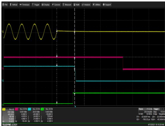
Figure 21: µMP10T-S2Q-S2Q-S2Q-S2Q-S2Q-S2Q-90-A Hold-up Time via AC mains Vin = 90Vac/63Hz Load: I O = 41.66A I SB = 2A Ch 1: AC Mains Ch 2: V SB Ch 3: V O Ch 4: Global DCOK
