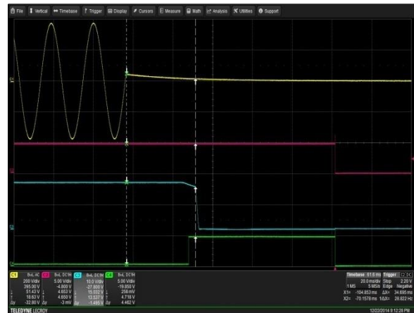
Figure 19: LCM600N Hold-up Time - V_{in} = 264VAC / 47Hz / 0^\circ
