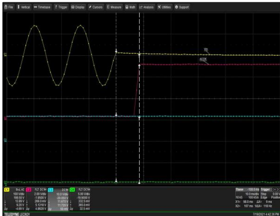
Figure 13: LCM600L ACOK Signal Turn-off Delay - V_{in} = 100VAC Load: I_o = 2A (12V), I_{SB} = 0A (5V) Ch 1: AC Mains Ch 2: ACOK Ch 3: Vo Ch 4: DCOK
