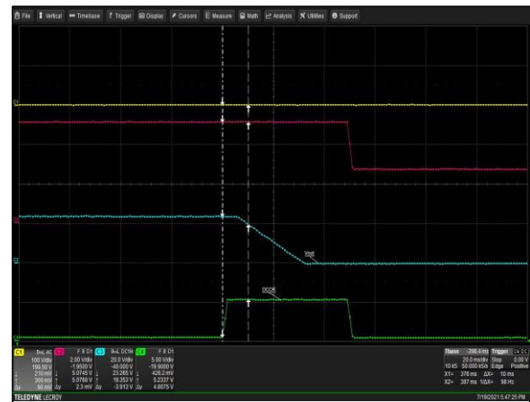
Figure 44: LCM600Q DCOK Signal Turn-off Delay - V_{in} = 100VAC
