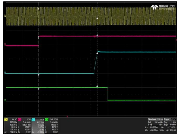
Figure 17: LCM600N Turn-on Delay via INH_EN - V_{in} = 90VAC
