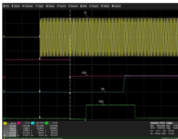
Figure 41: LCM600Q ACOK Signal Turn-on Delay - V_{in} = 100VAC Load: I_o = 2A (24V), I_{SB} = 0A (5V) Ch 1: AC Mains Ch 2: ACOK Ch 3: V_o Ch 4: DCOK
