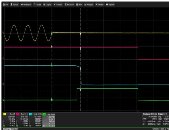
Figure 18: LCM600N Hold-up Time - V_{in} = 90VAC / 63Hz / 0^\circ
