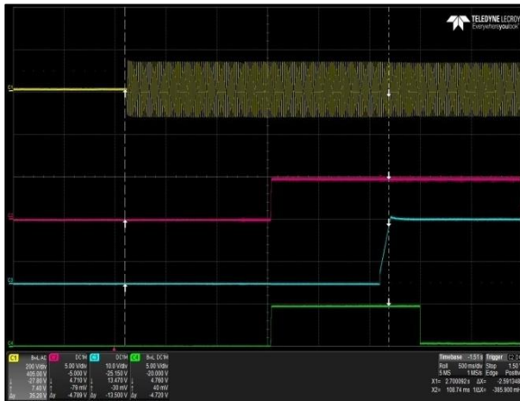
Figure 16: LCM600N Turn-on Delay via AC Mains - V_{in} = 90VAC
