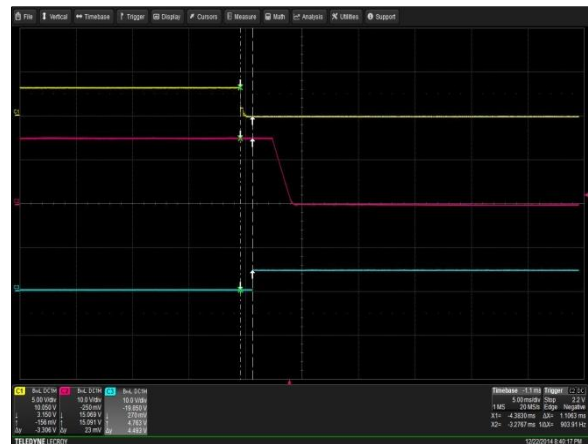
Figure 21: LCM600N Turn-off Characteristic via INH_EN
