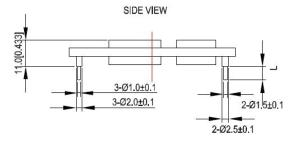
UNIT: mm[inch] BOTTOM VIEW: pin on upside TOLERANCE: X.Xmm±0.5mm[X.X in.±0.02in.]
