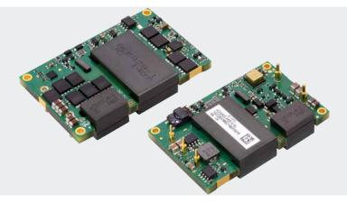
Advanced Energy's Artesyn ADQ600 series quarter-brick isolated DC-DC converter produces a single fully regulated 12 V output. Rated at 600 watts, the converter can deliver up to 50 amps output current and has no minimum load requirement. It has an input voltage range of 40 to 60 V and is primarily designed for use with standard 48 V supplies in computing and server applications, as well as regulated 48V supplies in telecommunications equipment.
