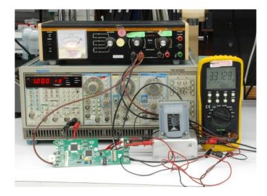
*Figure 3a - Typical voltage injection PSRR measurement test setup, utilizing a high current DC power supply. Using a DC power supply without an amplifier necessitates the use of additional equipment such as isolating components and external monitoring equipment.*
