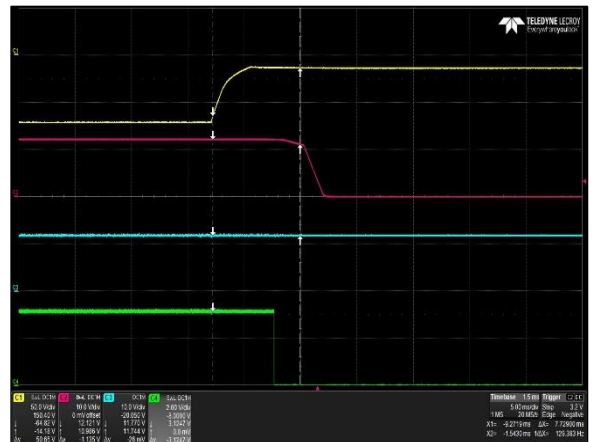
Figure 4: DS500SDC-3 Hold-up Time Vin = -72Vdc Load: I O = 41.6A I SB = 3A Ch 1: DC Mains Ch 2: V O Ch 3: V SB Ch 4: Pwr_Good
