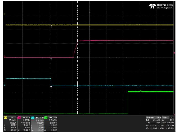
Figure 2: DS500SDC-3 Turn-On Delay via PS_ON Vin = -36Vdc Load: I O = 41.6A I SB = 3A Ch 1: DC Mains Ch 2: V O Ch 3: PS_ON Ch 4: Pwr_Good
