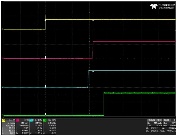
Figure 1: DS500SDC-3 Turn-On Delay via DC Mains Vin = -36Vdc Load: I O = 41.6A I SB = 3A Ch 1: DC Mains Ch 2: V O Ch 3: V SB Ch 4: Pwr_Good
