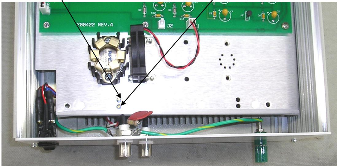
**POWER AMPLIFIER OFFSET/GAIN CALIBRATION Cont'd:****Figure 2 – Power Amplifier Offset/Gain Setup**
