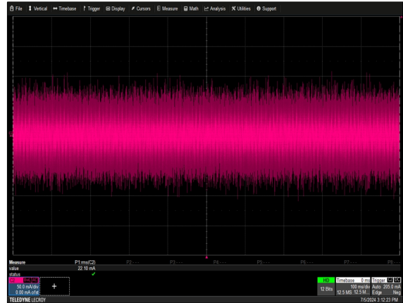
Figure 49: NP08W1-1MQ0-00-A-0 Ripple and Noise Measurement Load: R = 1.43 ohm Ch 2: I_O
