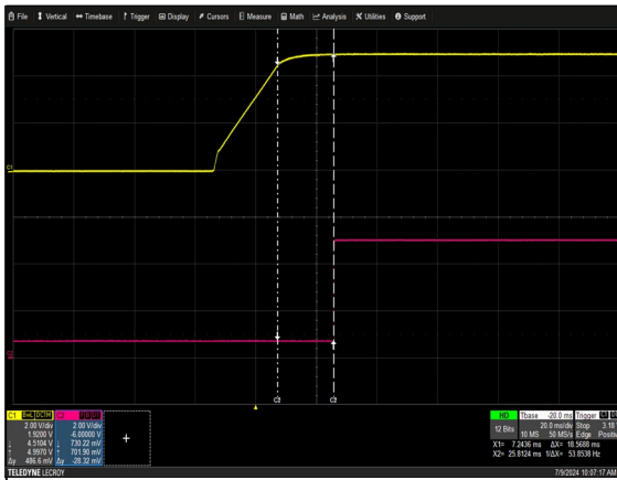
Figure 15: NP08W1-1ME0-00-A-0 Output Voltage Startup Characteristic Load: I_o = 56A Ch 1: V_O Ch 2: ISO_POWER_GOOD
