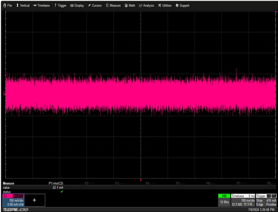
Figure 31: NP08W1-1ML0-00-A-0 Ripple and Noise Measurement Load: R = 0.36 ohm Ch 2: I_O
