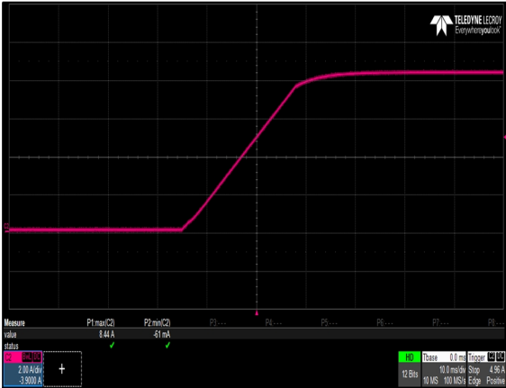
Figure 57: NP08W1-1MW0-00-A-0 Output Current Startup Characteristic Load: R = 5.78 ohm Ch 2: I_O
