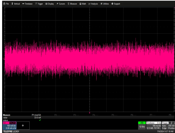
Figure 22: NP08W1-1ME0-00-A-0 Ripple and Noise Measurement Load: R = 0.08 ohm Ch 2: I_O
