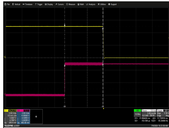
Figure 16: NP08W1-1ME0-00-A-0 Turn Off via Module Inhibit Load: I_o = 56A Ch 1: V_O Ch 2: Module Inhibit
