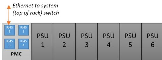
Multiple PSU shelves with one PMC per shelf connected:
