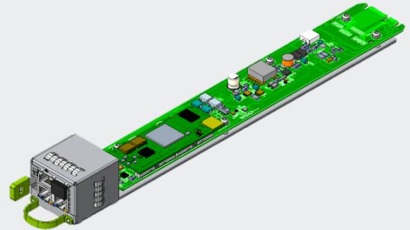
Advanced Energy's ORv3 HPR Power Management Controller (PMC) is a hot-pluggable controller in the shelf that monitors and facilitates the power supply units through a 10/100/1000MB Base-T Ethernet port and can be connected directly to the rack switch. The PMC communicates with PSUs in the shelf through its backplane connector. The front connector provides one Ethernet port and one RS232 port for debugging.
