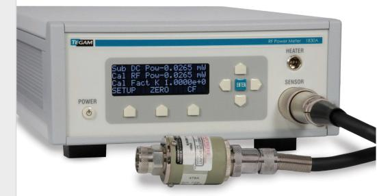
Thermistor RF power sensors are universally recognized as the most accurate means to measure and transfer RF power. The TEGAM Model 1830A was designed to operate with all types of thermistor RF power sensors while reducing uncertainties. It combines a modern DC substitution bridge with a precision measurement system to provide consistent, calibrated RF power readings manually or automatically.
