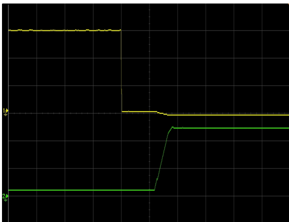
Figure 3: NDQ1300-48S12B-6LI Remote On Waveform (50ms/div) Vin = 50V Load: Io = 106A Ch 1: Remote On (1V/div) Ch 2: Vo (5V/div)
