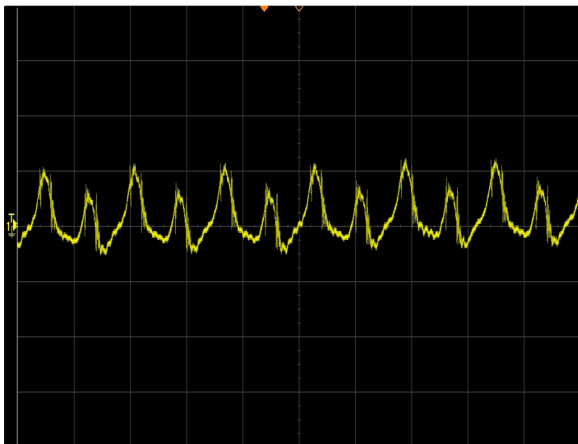
Figure 5: NDQ1300-48S12B-6LI Ripple and Noise (5μs/div) Vin = 50V Load: Io = 106A Ch 1: Vo (20mV/div)
