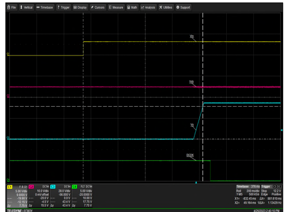
Figure 16: LCC1200-48U-9P Turn-on delay via INH_EN Vin = 264Vac Load: Io = 25A (48V), I SB = 1.5A (5V) Ch 1: INH_EN Ch 2: V SB Ch 3: V O CH 4: G_DCOK_C
