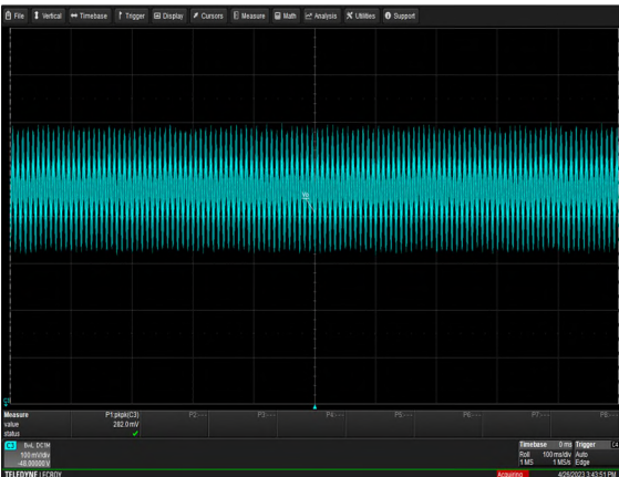
Figure 23: LCC1200-48U-9P Ripple and Noise Measurement Vin = 230Vac Load: Io = 25A (48V), I SB = 1.5A (5V) Ch 1: V O
