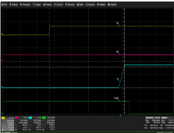
Figure 15: LCC1200-48U-9P Turn-on delay via INH_EN Vin = 90Vac Load: Io = 16.67A (48V), I SB = 1.5A (5V) Ch 1: INH_EN Ch 2: V SB Ch 3: V O CH 4: G_DCOK_C
