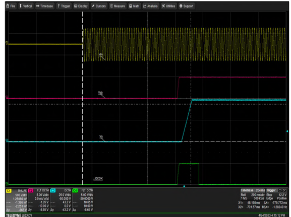
Figure 14: LCC1200-48U-9P Turn-on delay via AC mains Vin = 264Vac Load: Io = 25A (48V), I SB = 1.5A (5V) Ch 1: AC Mains Ch 2: V SB Ch 3: V O CH 4: G_DCOK_C
