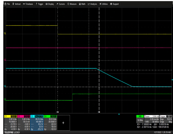
Figure 8: LCC1200-28U-9P Turn Off Characteristic via INH_EN Load: I_o = 42.9A (28V), I_{SB} = 1.5A (5V) Ch 1: INH_EN Ch 2: V_{SB} Ch 3: V_o Ch 4: G_DCOK_C
