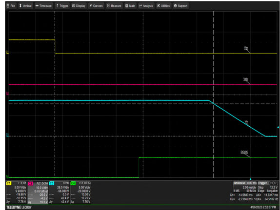
Figure 20: LCC1200-48U-9P Turn Off Characteristic via INH_EN Load: Io = 25A (48V), I SB = 1.5A (5V) Ch 1: INH_EN Ch 2: V SB Ch 3: V O CH 4: G_DCOK_C
