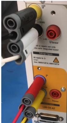
*Figure 5: CA-70-5 and CA-71-5 connections to Power Analyzer*
