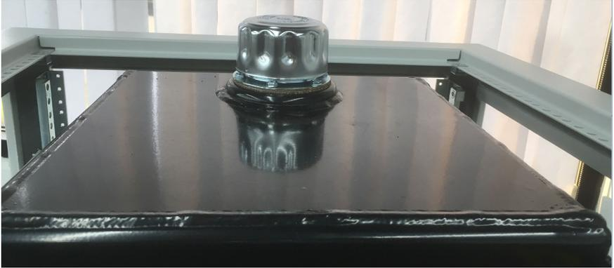
Figure 3: 1 kW Chiller coolant reservoir
