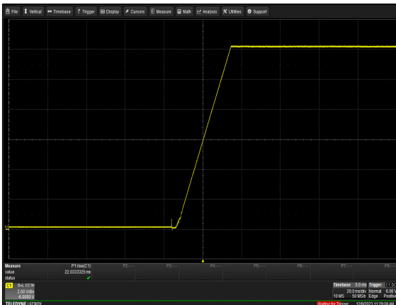
Figure 9: CSU1600AT-3-100 Output Voltage Startup Characteristic V_{in} = 90V_{ac} Load: I_o = 81.9A I_{SB} = 3.5A Ch 1: V_O
