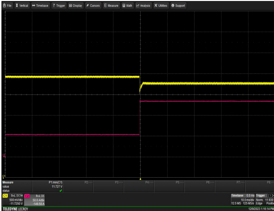
Figure 11: CSU1600AT-3-100 Transient Response - V_O Deviation 40% to 100% load change 1A/ \mu S slew rate V_{in} = 230V_{ac} Ch 1: V_O Ch 2: I_O Output Cap: 2200uF
