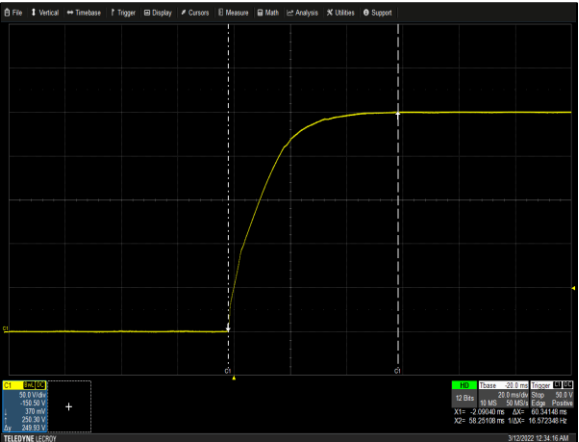
Figure 5: LCM4000HV-T Output Startup Characteristic Vin = 311VAC Load: Io = 16A Ch 1: Vo
