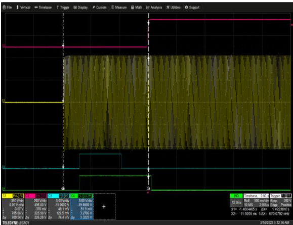
Figure 2: LCM4000HV-T Turn-on delay via AC mains Vin = 520VAC Load: Io = 16A Ch 1: Vin Ch 2: Vo Ch 3: AC_OK Ch 4: DC_OK
