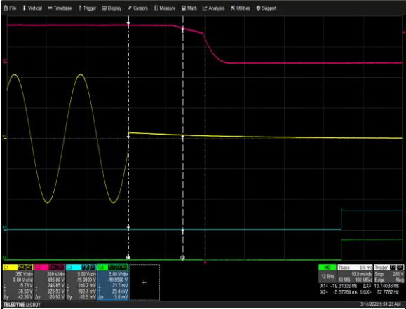
Figure 4: LCM4000HV-T Hold-up Time Vin = 520VAC Load: Io = 16A Ch 1: Vin Ch 2: Vo Ch 3: AC_OK Ch 4: DC_OK
