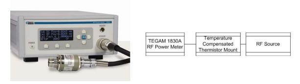
Figure 3 - TEGAM 1830A Method for Measuring Thermistor Mounts
