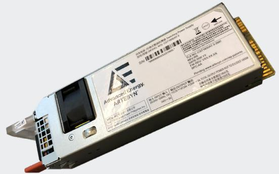
Advanced Energy's Artesyn CST1800AT front end series is designed to provide a flexible power conversion solution for compute, storage, and networking equipment in the modular hardware common redundant power supply (M-CRPS). The 1800 W model is in the smaller form factor of 1 U x 60 mm x 185 mm. The series of power supply can cover cost-sensitive entry level systems, or power hungry applications where there are space constraints.
