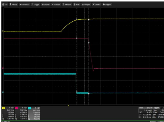
Figure 45: CSU2000AP-3-211 Turn Off Characteristic via PS ON Load: I_o = 163.9A I_{SB} = 3.5A Ch 1: PS ON Ch 2: V_O Ch 3: PWOK
