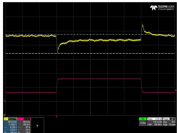
Figure 10: CSU2000AP-3-100 Transient Response - V_O Deviation 40% to 100% load change 0.5A/\mu s slew rate V_{in} = 230V_{ac} Ch 1: V_O Ch 2: I_o
