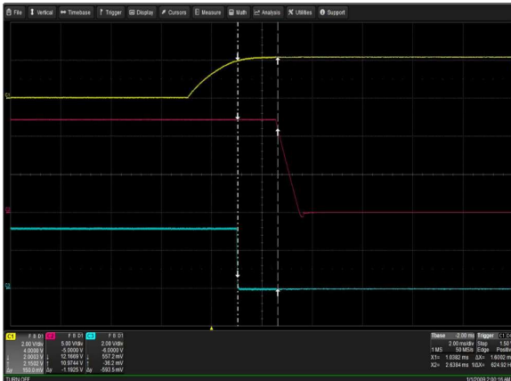
Figure 21: CSU2000AP-3-111 Turn Off Characteristic via PSOK Load: I_o = 163.9A I_{SB} = 3.5A Ch 1: PSOK Ch 2: V_O Ch 3: PWOK
