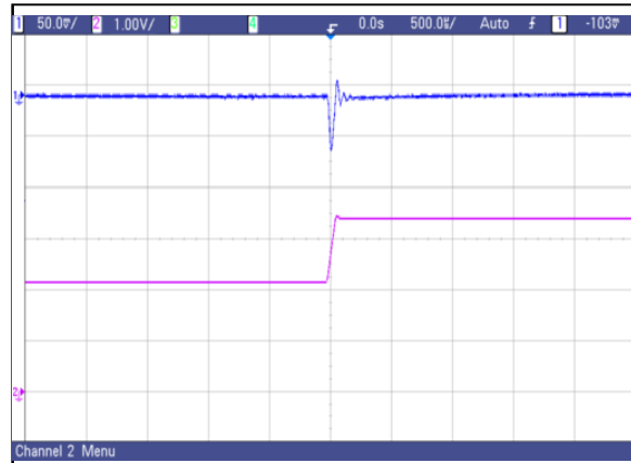
Figure 6: AVO75-48S1V2 Transient Response 50%-75% load change, 0.1A/uS slew rate, Vin=48V
