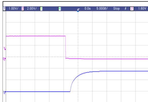
Figure 26: AVO75-48S1V8 typical start-up from CNT on
