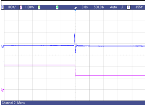
Figure 29: AVO75-48S1V8 Transient Response 50%-25% load change, 1A/uS slew rate, Vin=48V Ch 1: Vo Ch 2: Io
