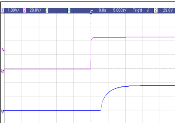
Figure 25: AVO75-48S1V8 typical start-up from power on
