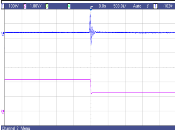
Figure 7: AVO75-48S1V2 Transient Response 50%-25% load change, 1A/uS slew rate, Vin=48V Ch 1: Vo Ch 2: Io
