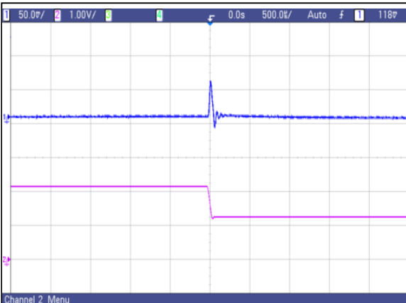
Figure 5: AVO75-48S1V2 Transient Response 50%-25% load change, 0.1A/uS slew rate, Vin=48V
