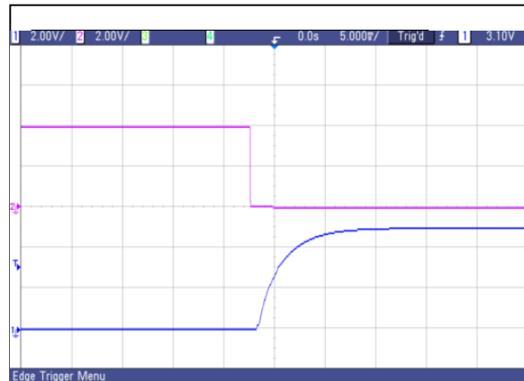
Figure 59: AVO75-48S05 typical start-up from CNT on
