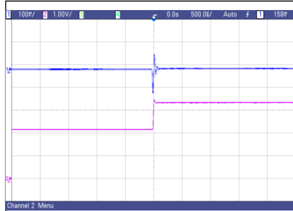
Figure 30: AVO75-48S1V8 Transient Response 50%-75% load change, 1A/uS slew rate, Vin=48V Ch 1: Vo Ch 2: Io
