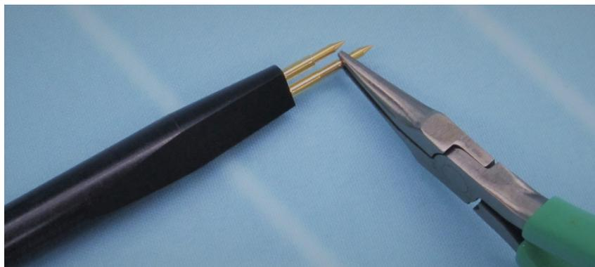
2. To fully install the new pin, position the new pin in the socket and press it against a hard surface.
