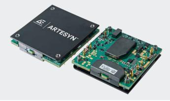
Advanced Energy's Artesyn AVE700-48S28PB-6L is a single output DC/DC converter with standard half-brick outline and pin configuration. It delivers up to 25A output current with 28V output. Ultra-high 95.5% efficiency and excellent thermal performance makes it an ideal choice for use in computing and telecommunication applications and can operate over an ambient temperature range of -40 °C ~ +85 °C. without air cooling, and baseplate operating temperature up to 100 °C.
