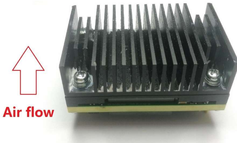
Figure 16 Typical test condition, heatsink
