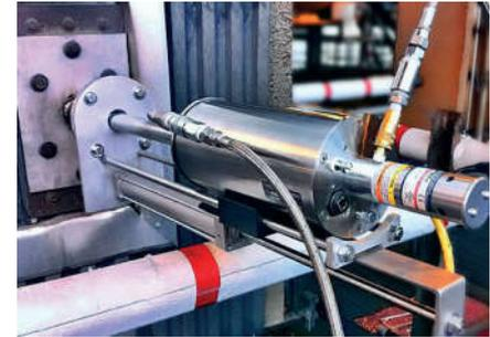
▲ Fig 4. (small) Specially designed camera retraction system.
