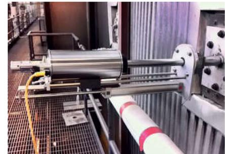
▲ Fig 5. Specially designed camera retraction system [2].
