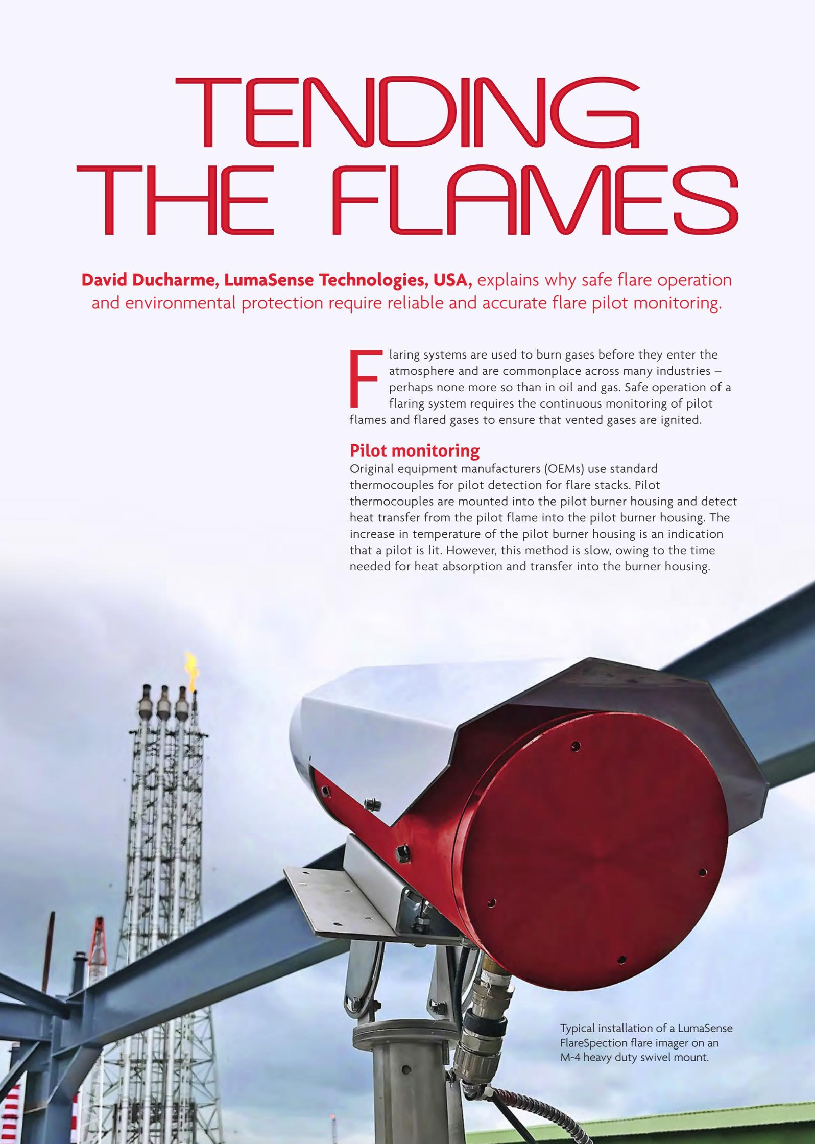
Typical installation of a LumaSense FlareSpection flare imager on an M-4 heavy duty swivel mount.
