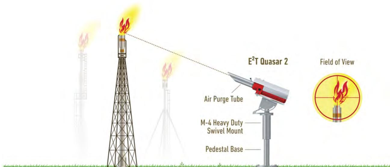
**Figure 1.** Flare monitoring systems are located at a distance about equal to the height of the flare stack to get a proper field of view.
