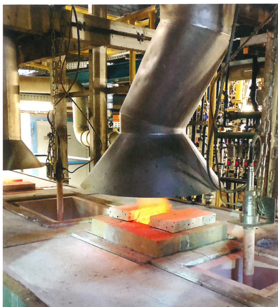
IMPAC IS 50-LO/GL pyrometer with an Inconel sighting tube in a glass forehearth.
