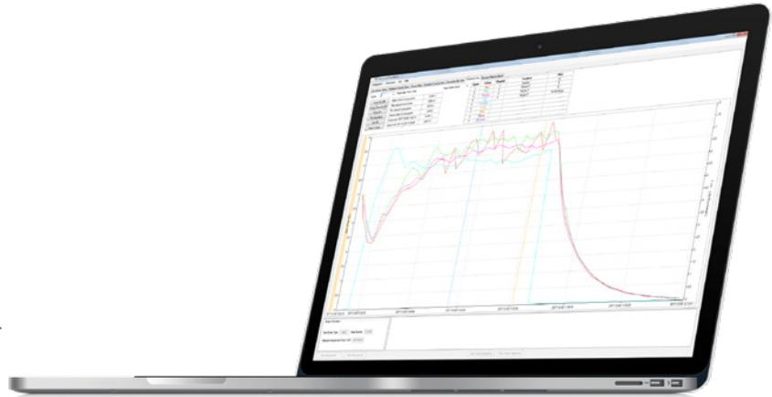
The Advanced Ventilation Software 7651 from LumaSense Technologies enables remote control of a 1512 or a 1412i Photoacoustic Gas Monitor and a 1403 Multipoint Sampler and Doser unit. The software coordinates the functions of the instruments to form a monitoring system which, via tubing, can perform ventilation and air exchange measurements. The system can also perform gas-monitoring tasks in up to 6 different locations.
