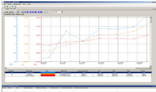
Fig. 1: The graphical window shows up to seven graphs. The user selects the data plotted, the scaling, and the style and color of the lines and background to build the graphical window.
