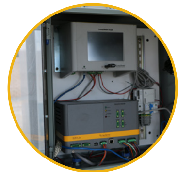
Separate supporting electronics can be mounted up to 30 meters away in a separate enclosure. This allows for a compact sensor that can be conveniently mounted anywhere.
